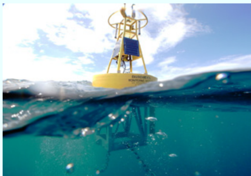
This coastal buoy supports a full array of water quality sensors, data acquisition systems, and meteorological sensors. Its hull and structure are rugged enough to withstand significant wind and wave activity in ocean applications in less than 75 meters of water depth.
