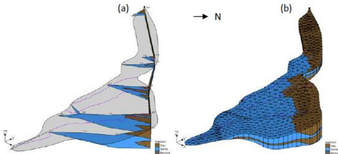
Figure 1: (a) Cross-sections created based on borehole data for the coastal aquifer of Guyana and (b) the interpolated 3D solid using GMS MODFLOW
