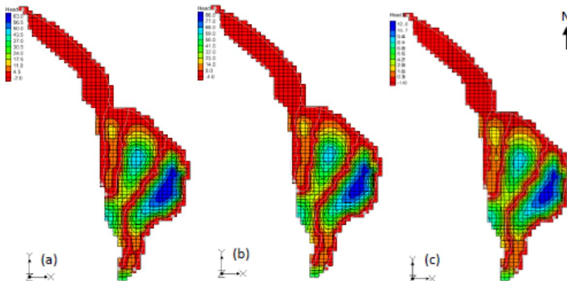
Figure 3: Model output with the estimated recharge rates (m d<sup>-1</sup>): (a) R=0.0027 (b) R=0.0036 (c) R=0.0005
