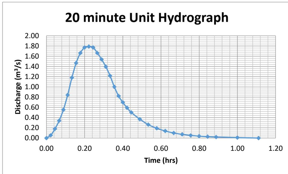
Figure 3 Twenty minute unit hydrograph
