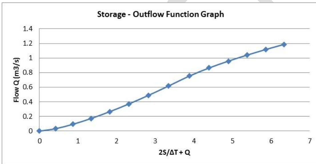
Figure 2: Storage-Outflow Function
