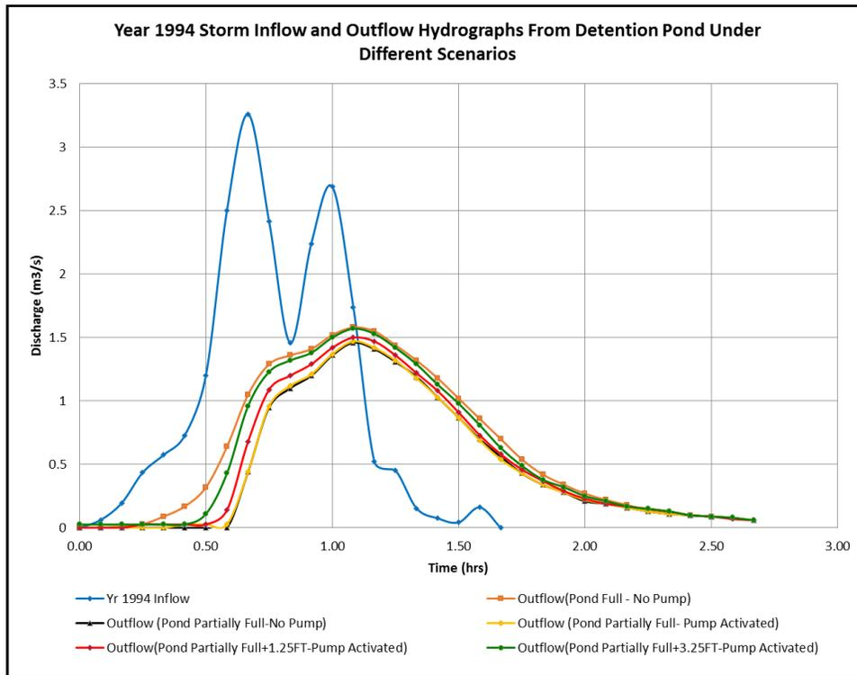
Figure 5: Simulated performance of the FERP for various scenarios.
