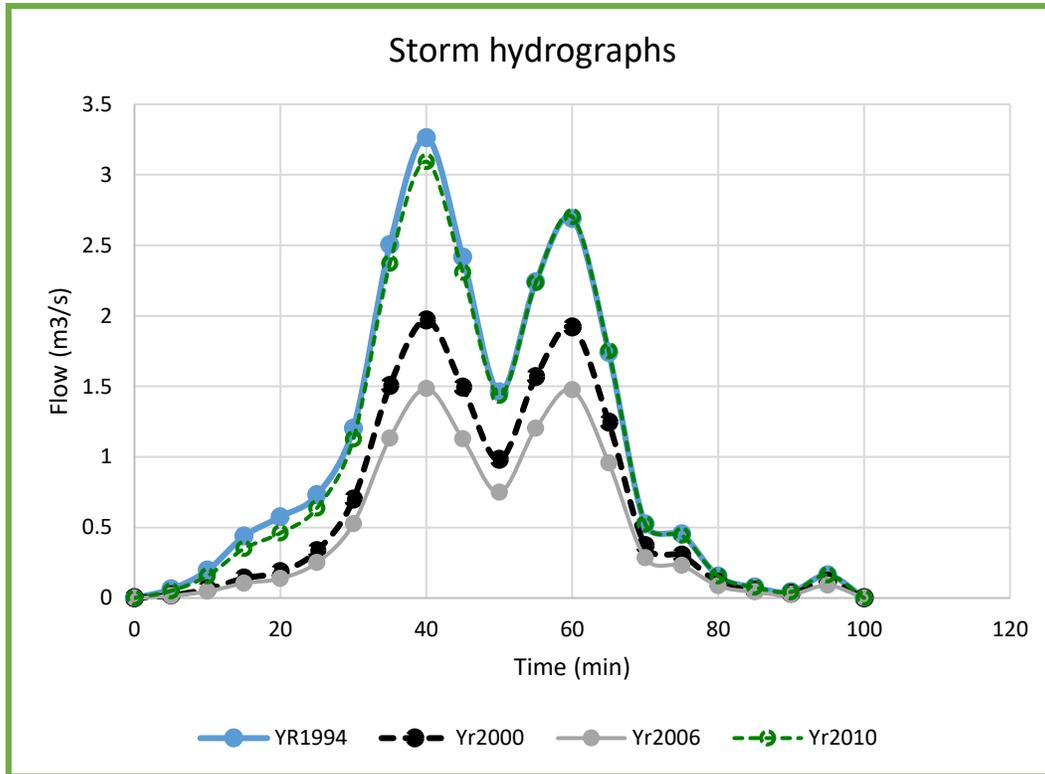
Figure 4: Simulated Storm Hydrograph for historic extreme storms
