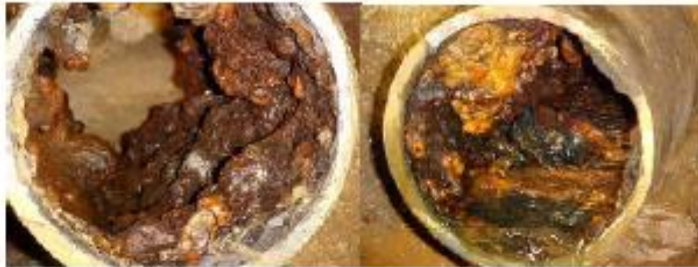
Figure 2.10: Cast Iron Pipe Sections Replaced
