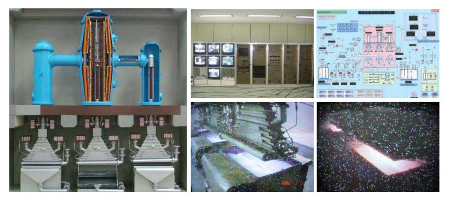
Full-scale application of electron beam wastewater treatment plant for 10,000 m<sup>3</sup>/d of textile dyeing wastewater with 1 MeV, 400 kW accelerator.
