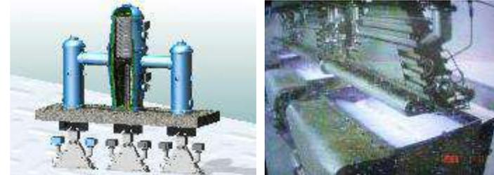
Commercial plant for treating textile dyeing wastewater (1,000 m<sup>3</sup>/d), Rep. of Korea
