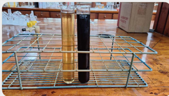
Figure 2. Visual comparison of Constructed Wetland treated leachate (left test tube) vs untreated leachate (right test tube) November 2024
